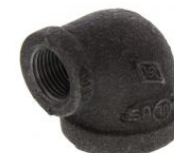
3/4" x 3/8" Black Malleable Reducing 90 Degree Elbow
