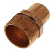
1-1/4" Female Copper Solder x 1-1/2" Male NPT Adapter
