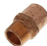
1" Female Copper Solder x 3/4" Male NPT Adapter
