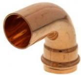
1-1/4" Copper Press-Fit Street 90 Elbow
