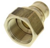
1" Female NPT x 3/4" F1960 Brass Expansion PEX Adapter (Lead Free)
