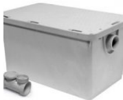
Endura25XT 50 lb Capacity, 25 GPM Grease Trap (2" Connection)
