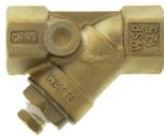
1" Female NPT Bronze Wye Strainer (Lead Free)
